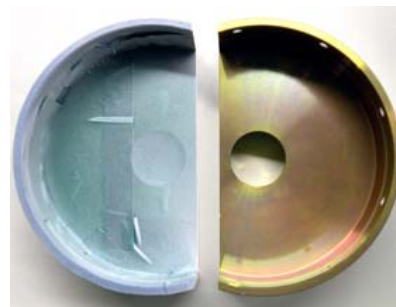
Chem film is sometimes applied to help masking adhere to a part before anodizing .
